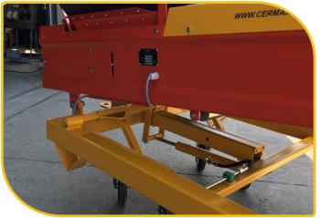
Features: hydraulically adjustable infeed height, retractable drawbar
