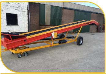
**Features:** rubber chevron belt with high flights, two-speed gear motor as standard
