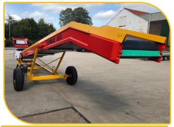
**Option:** main wheels that can turn perpendicular to conveyor, with electrically driven main wheel
