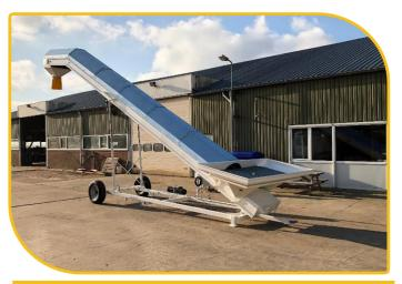
**Option:** large infeed hopper with filling grid and pricker, belt cover made of galvanized sheet, discharge chute with flap
